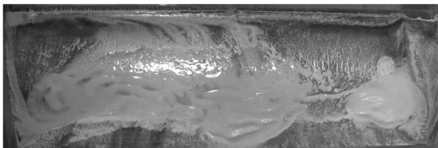
Fig. 10 Experimental and numerical pressure coefficient distributions, AOA = 14 deg, Re = 150,000 . The lower inset shows titanium dioxide rendered skin friction patterns.
